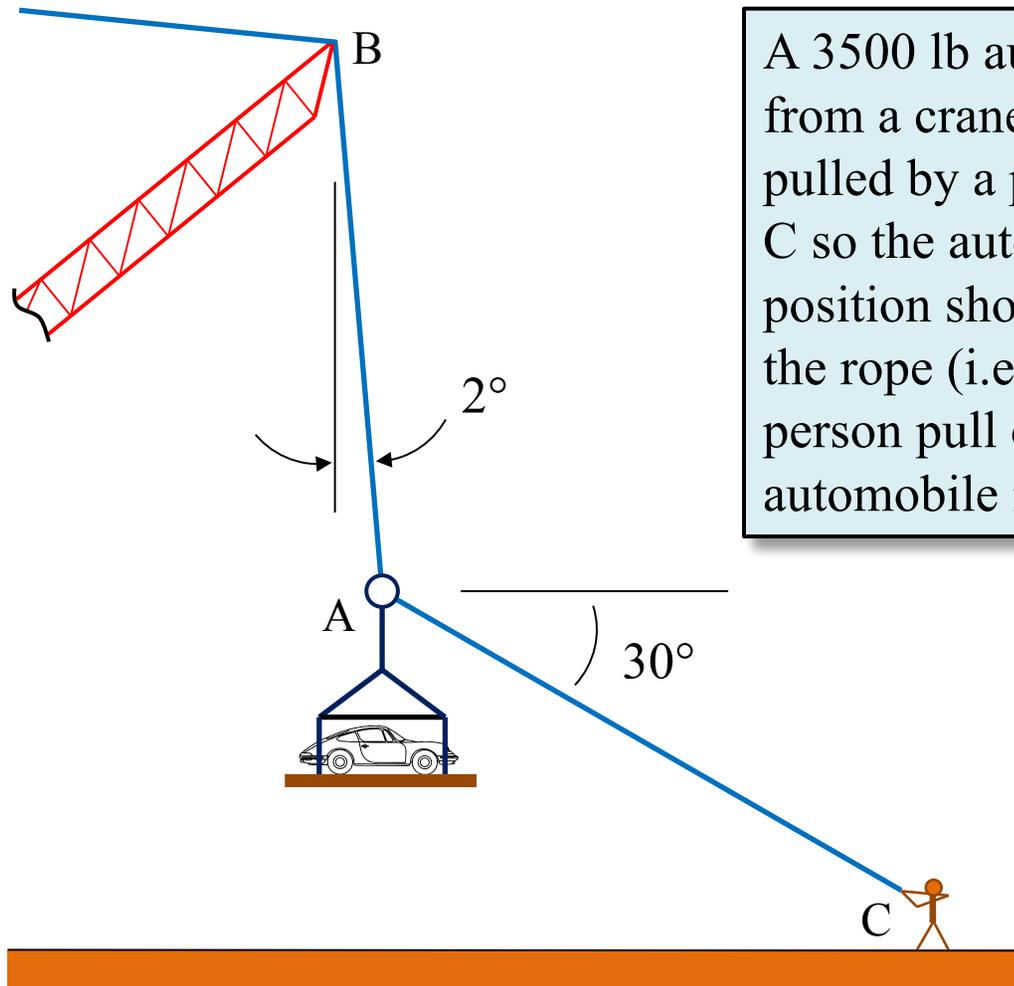
A 3500 lb automobile is suspended from a crane. The support at A is pulled by a person with a rope at point C so the automobile is held in the position shown. What is the tension in the rope (i.e. how hard must the person pull on the rope to hold the automobile in the position shown)?
